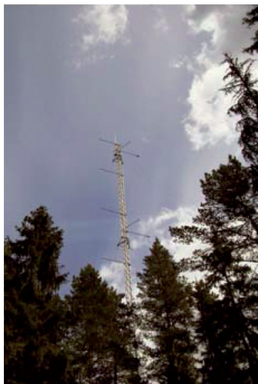
Comprehensive ecosystem measurement site in Norunda, Sweden. The tower measures the amount of CO 2 exchanged between the forest and the atmosphere.
